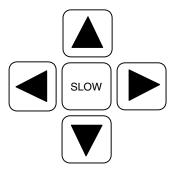
Press the left and right slew keys to unroll material before plotting, to position the tool for plotting, to position the carriage and material between jobs, and to rotate the drum and feed material through the plotter or back toward the roll holder.
